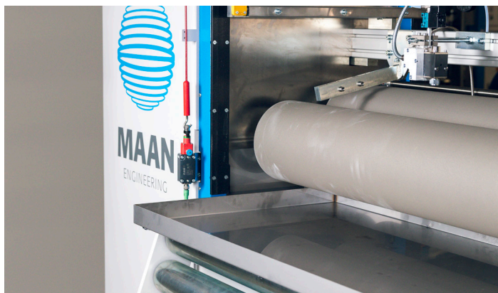
Drip tray and steel, oil heated, rollers
