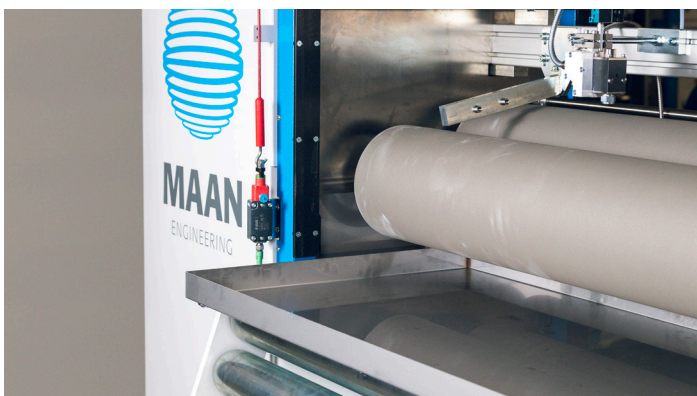
Drip tray and steel, oil heated, rollers
